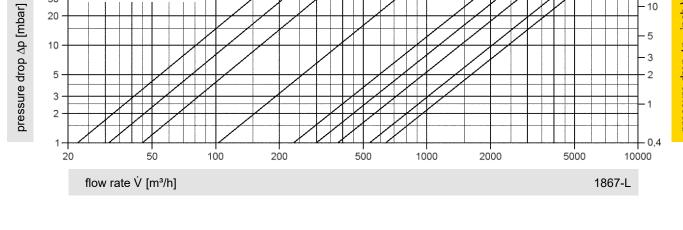
The flow capacity charts have been determined with a calibrated and TÜV certified flow capacity test rig. Volume flow V in (m³/h) and CFH refer to the standard reference conditions of air in ISO 6358 (20°C, 1bar). For conversion to other densities and temperatures, refer to Sec. 1: "Technical Fundamentals."
