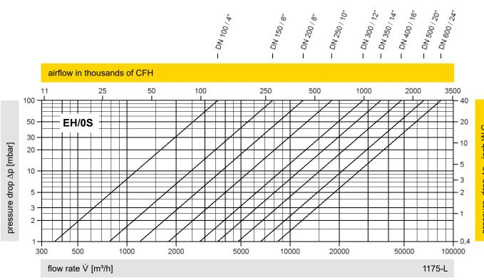
The flow capacity charts have been determined with a calibrated and TÜV certified flow capacity test rig. Volume flow  $\dot{V}$  in (m³/h) and CFH refer to the standard reference conditions of air in ISO 6358 (20°C, 1bar). For conversion to other densities and temperatures, refer to Sec. 1: "Technical Fundamentals."
