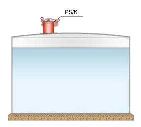
Gauge hatches can be welded onto tanks with floating roof.
