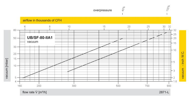
The flow capacity charts have been determined with a calibrated and  $T\ddot{U}V$  certified flow capacity test rig. Volume flow  $\dot{V}$  in (m³/h) and CFH refer to the standard reference conditions of air in ISO 6358 (20°C, 1bar). For conversion to other densities and temperatures, refer to Sec. 1: "Technical Fundamentals."
