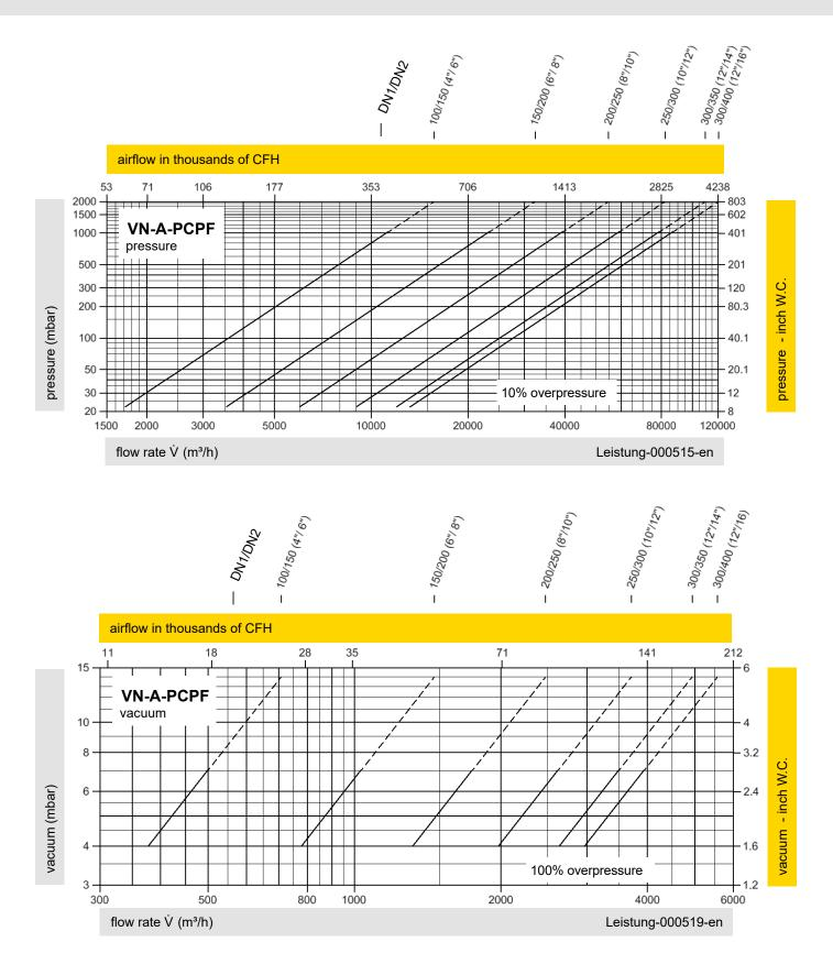
The flow capacity charts have been determined with a calibrated and TÜV certified flow capacity test rig. Volume flow  $\dot{V}$  in (m³/h) and CFH refer to the standard reference conditions of air in ISO 6358 (20°C, 1bar). For conversion to other densities and temperatures, refer to Sec. 1: "Technical Fundamentals."
