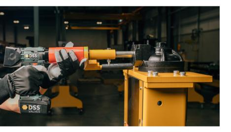
Torque-Tek was designed with efficiency in mind. It provides quick and easy actuation for large diameter valves that can take hours to operate, tedious projects with many small valves, and/or remote locations with few human operators.
