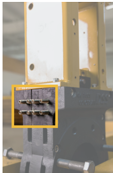
Figure 2: DBB (8) packing screws per side.
