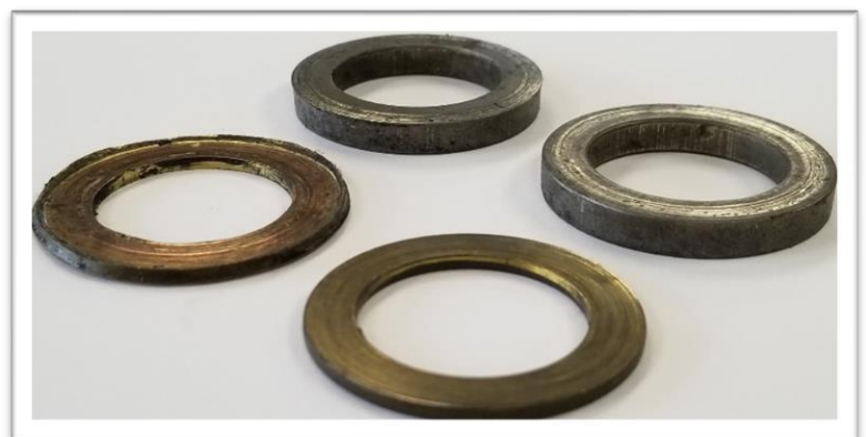
Figure 2: Premature Bearing Wear
